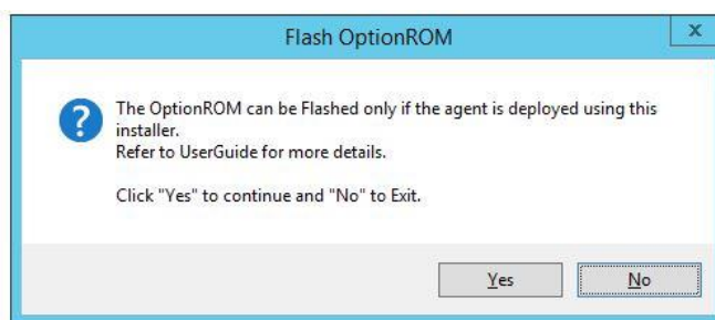
Figure 54 - Starting option ROM flashing
