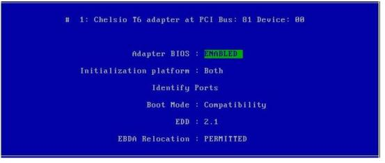
ONOTE Use the default values for Boot Mode, EDD and EBDA Relocation parameters, unless instructed otherwise. v. Choose **PXE** from the list to configure. Hit [Enter].
